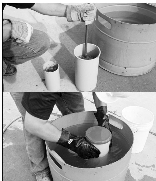
Making and Curing Cylinders in the Field
